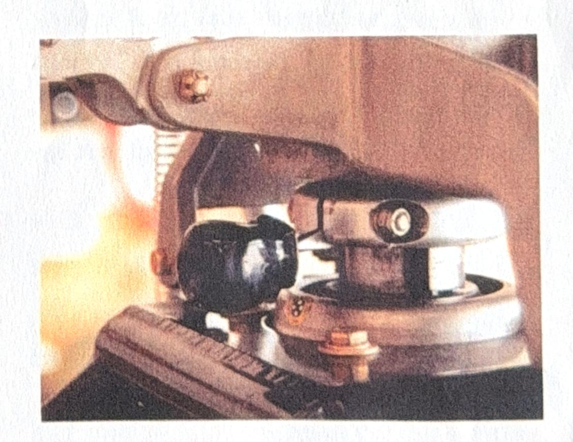
3. ☐ Snip and remove the Plastic Wire Tie (Tyrap) from the top of the Dust Boot. ✓
