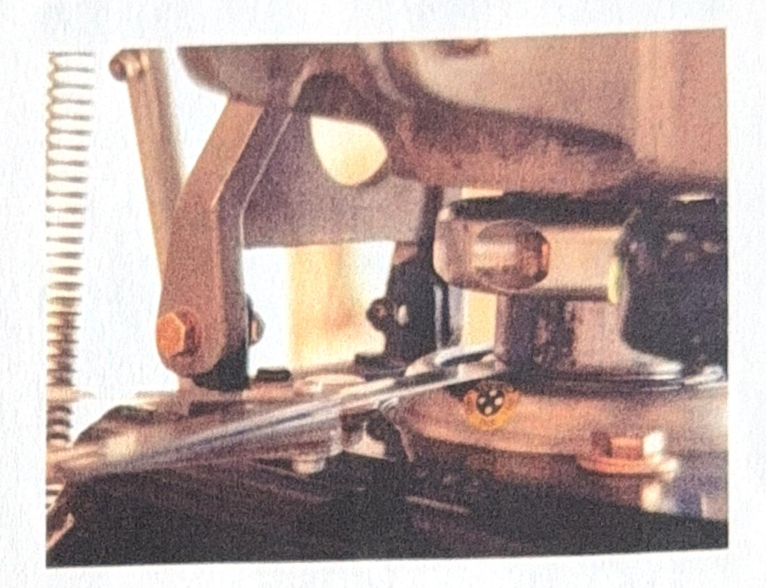
2. Remove the bolt and nut from the Sliderball Adjustment Collar and insert the tip of a "stubby" screwdriver into the slot in the collar and drive it in just enough to spread the slot to loosen the collar on the Sliderball.
